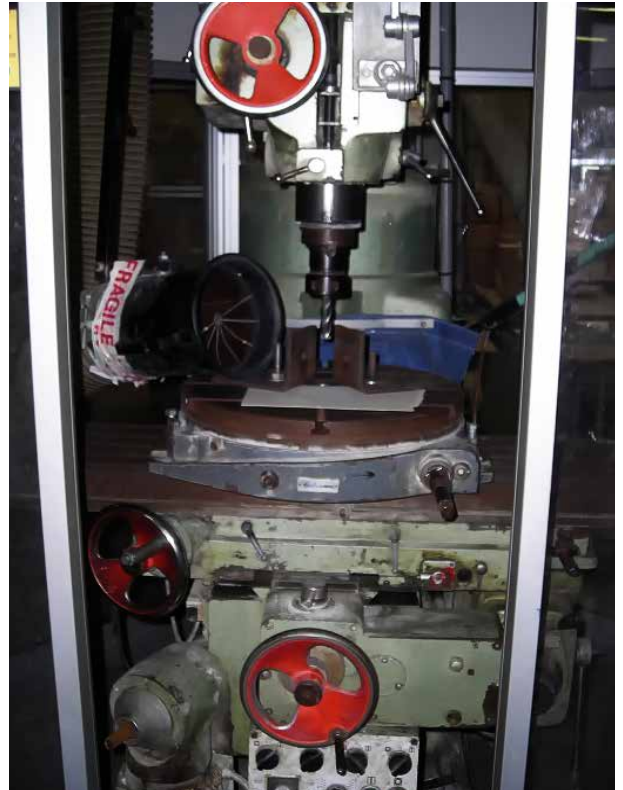
Drill with limited dust control
