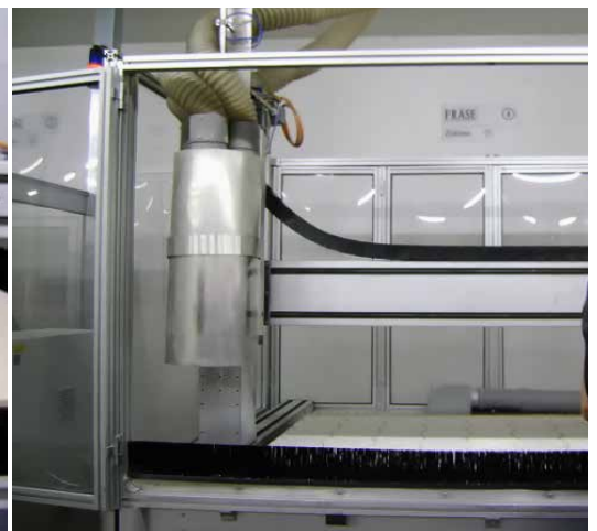
CNC with partial enclosure and LEV on tool
