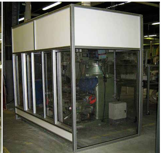
Router fully enclosed
