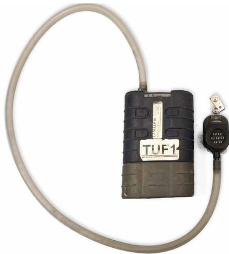
Fig. 3: Sampling assembly UKEA head (total dust)
