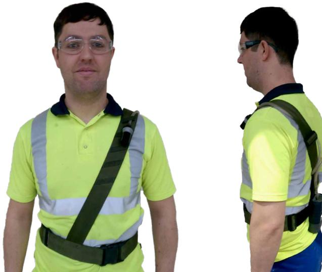
Fig. 1 & 2: Personal air sampling unit for airborne fibres
