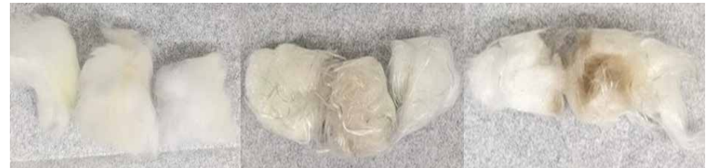
Figure 2 – Fibres post-exposure for “normal” conditions: quartz wool (left), insulation 1 (middle), and insulation 2 (right).
